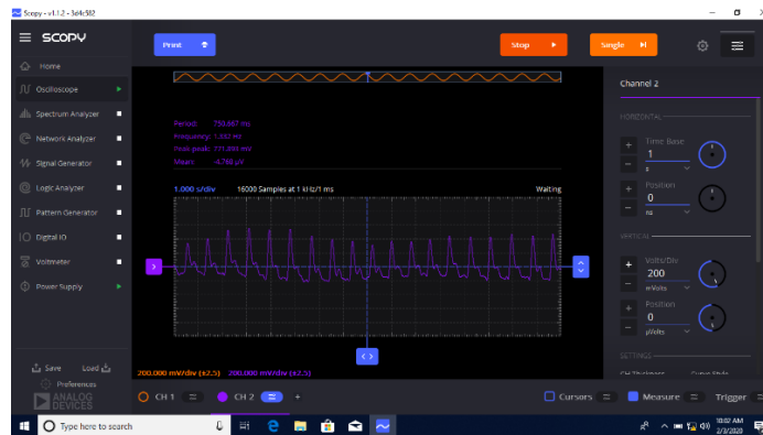
Figure 2: Screenshot for Scopy software interface displaying pulses in real time using an oscilloscope
